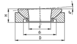
$\begin{array}{lll} D & = 32 \\ d & = 13 \\ d1 & = 20 \\ H & = 10 \\ Max \ screw \ dimension = M10 \\ Static \ load \ (kN) & = 43.4 \\ Weight \ (g) & = 44 \\ \end{array}$
